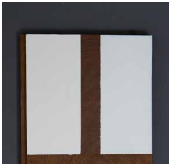
Figure 2. Wood with insulator treatment (Mowilith® SB 1000)
