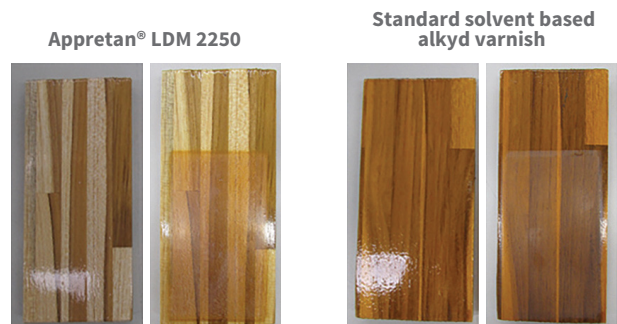
Before and after 1.200 hours of QUV exposition according to Norm ABNT NBR 15380 - condition 2
